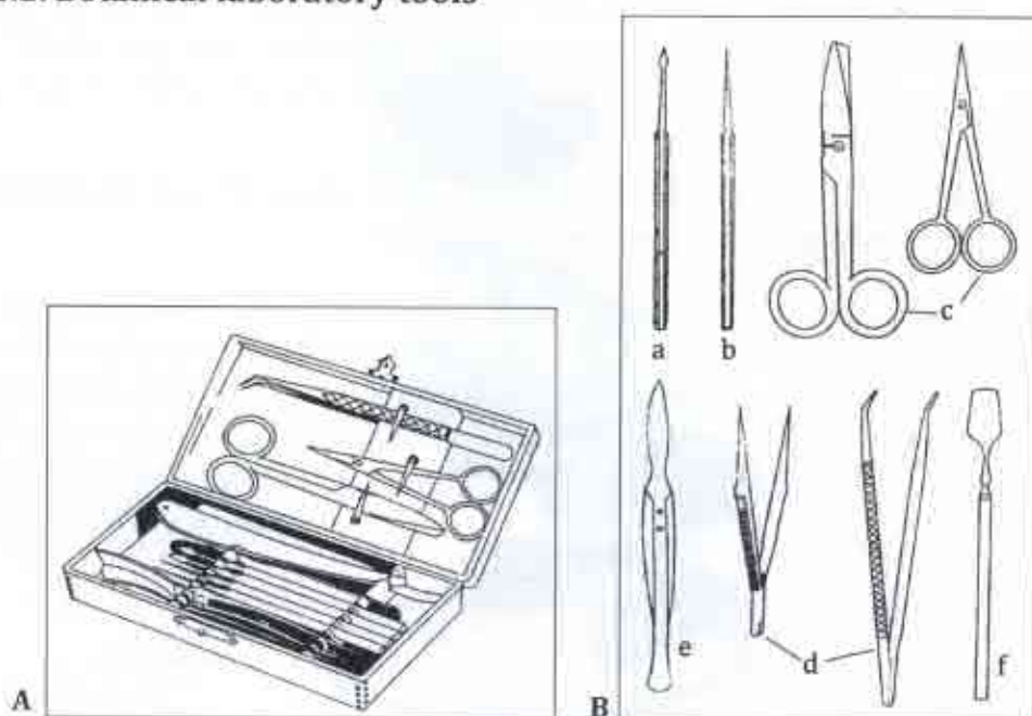
Fig. 4. Botanical laboratory tools: A – Box with microscopic utensils; B – necessary botanic laboratory tools: a – lanceolate preparation needle; b – pointed preparation needle; c – scissors; d – tweezers; e – scalpel; f – spatulate needle
