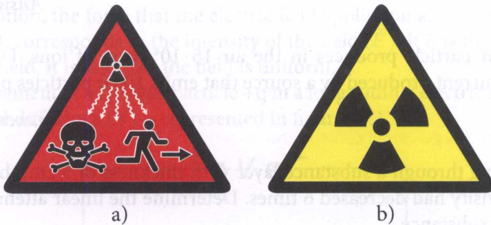
Fig. 18.5: a) new hazard warning symbol for highly radioactive elements; b) hazard warning symbol of radioactive substances stored in protective containers.
