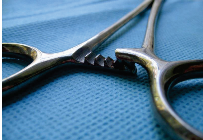
Fig.9. The rack type locking mechanism of surgical clamp, located from inside of the arms.
