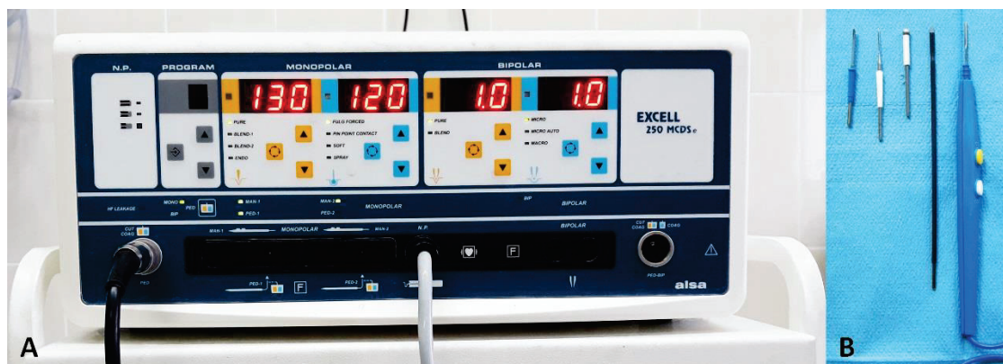
Fig.28. Electrosurgical equipment for diathermocautery during surgery: A. Electrosurgical power supply unit, which provides two modes of tissue exposure; B. Disposable plastic handle with attachable accessories of various shapes and lengths.
