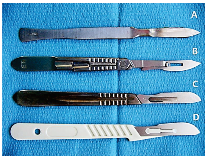
Fig.1. Surgical scalpels: A. Conventional scalpel, in which the handle and blade are unit in a common body; B.-C. Modern scalpels with a disposable and replaceable blade attached to a reusable handle; D. Completely disposable scalpel with plastic handle.
